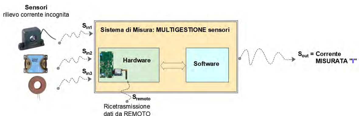
Figure 2: Different sensors applied to a single system, produces an identical result
