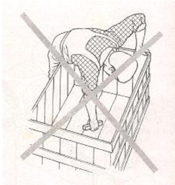
Figure 1. Bin at a working height where the worker has to bend to reach a far object Source: Kroemer et al, Ergonomics: How to Design for Ease and Efficiency (Fig. 11-17, p 540)
